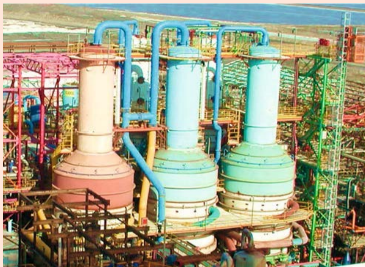
Fig. 6: Veolia's PIC™ Draft Tube Baffle HPD® crystallisers.
