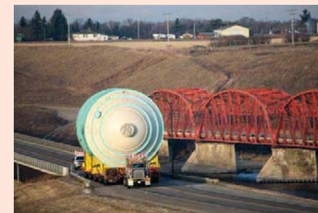
Fig. 5: Veolia's KCl crystalliser being transported to the project site.
