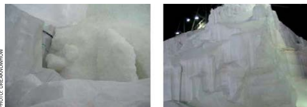
Fig. 1: Urea lumps (left) and severely caked storage pile (right).
