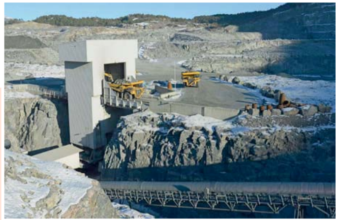
Direct-feed semi-mobile crushing plant at Norsk Stein, Norway.
