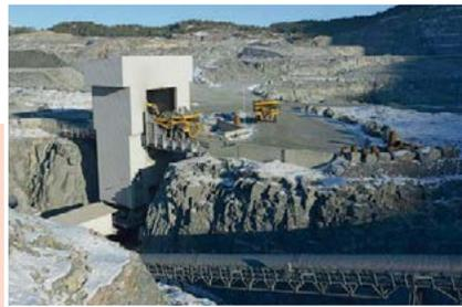
Direct-feed semi-mobile crushing plant at Norsk Stein, Norway.
