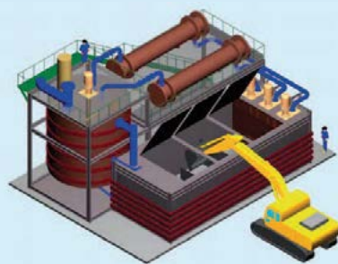
Fig 1: New Wales melter schematic. Rectangular pump tank, cylindrical melter mixing tank and tube-shaped heat exchangers.
