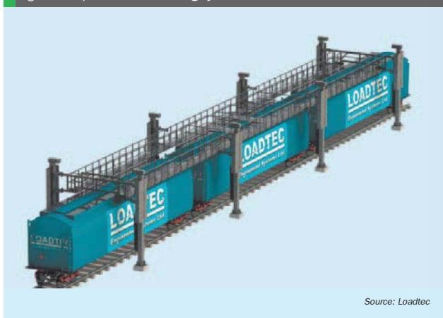
Fig 3: Carbis/Loadtec urea loading system for rail cars
