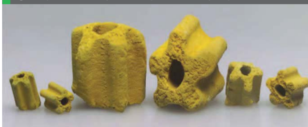
Fig 1: Sulphuric acid catalysts from Topsøe in the Daisy shape
