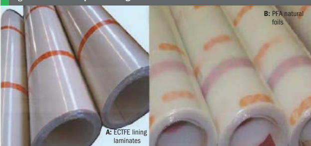
Fig 4: Fluoro-thermoplastic lining materials
