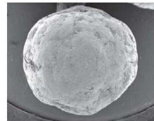
Above left: To be avoided: crystal bridge formation of a urea granule. Above centre and above right: Urea granules and prills after coating.
