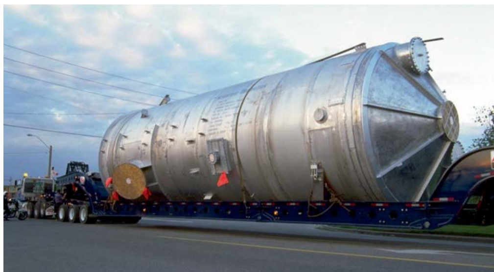
Fig. 3: Fully fabricated SARAMET® alloy acid tower.
