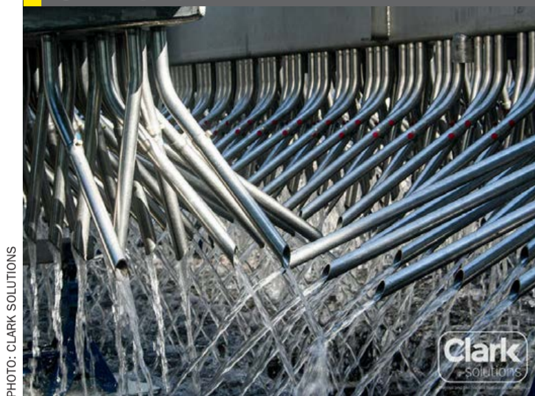
Fig. 2: Trough liquid distributor with downcomers in CSX™
