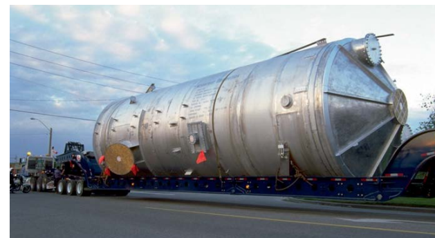
Fig. 3: Fully fabricated SARAMET® alloy acid tower.
