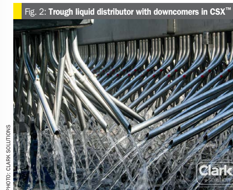
Fig. 2: Trough liquid distributor with downcomers in CSX™
