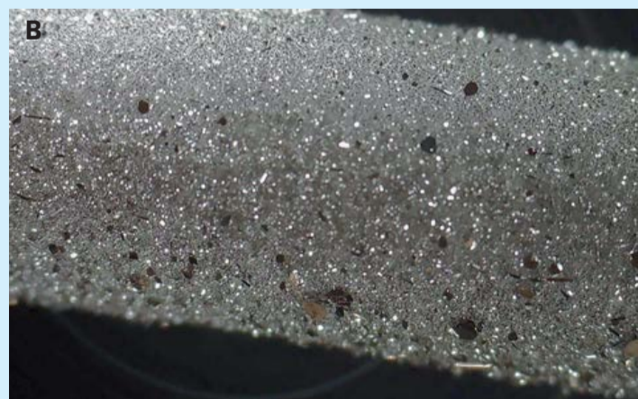
Fig. 1: Effects of platinum oxide sublimation. The thermocouple element thins to a needle point and platinum deposits up the ceramic element support as crystals. A) Mass loss thinning as a result of platinum oxidation. The bottom wire has full cross section remaining. B) Platinum crystals deposited on a ceramic element support.
