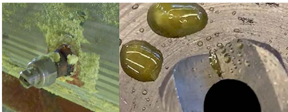
Fig. 3: Unheated nozzles (left) can be prone to plugging; heated nozzles (right) stay clear.
