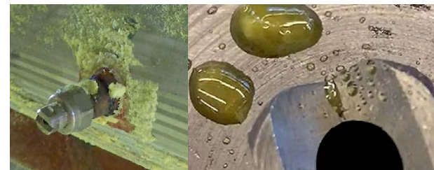
Fig. 3: Unheated nozzles (left) can be prone to plugging; heated nozzles (right) stay clear.
