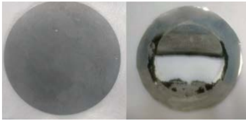
Fig. 5: 316L plate (Left: in acid/inert fluid system. Right: in acid/water system – a hole was used to mix fluids representing a mild leak.)
