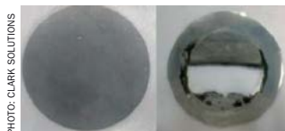
Fig. 5: 316L plate (Left: in acid/inert fluid system. Right: in acid/water system – a hole was used to mix fluids representing a mild leak.)
