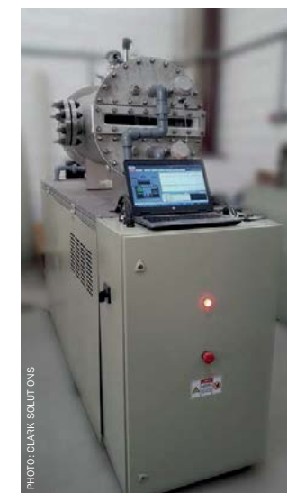
Fig. 6: SAFEHX physical experimental bench.
