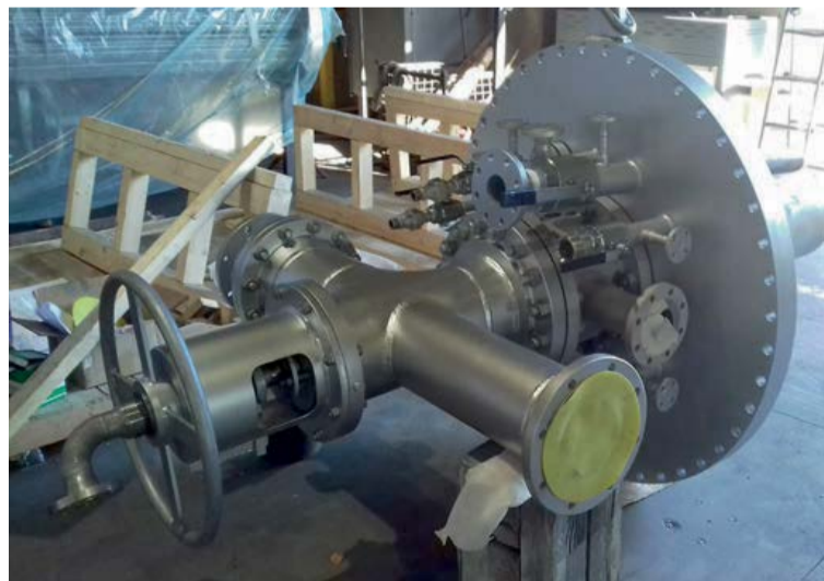
Fig. 4: Oxygen enrichment Claus burner
