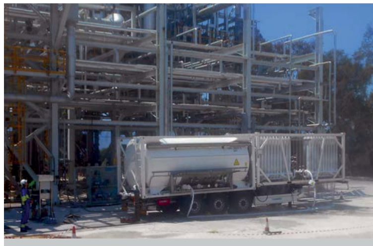
Fig. 2: Mobile oxygen supply chain based on liquid oxygen.
