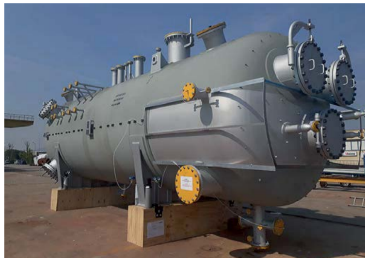
Fig. 5: New waste heat boiler (rear view)
