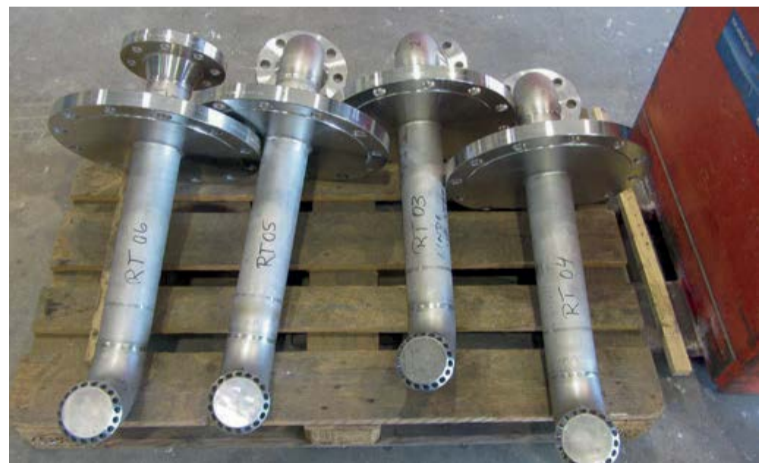
Fig. 3: Oxygen injectors OXYMIX™, tailor designed for Neste's Porvoo refinery.
