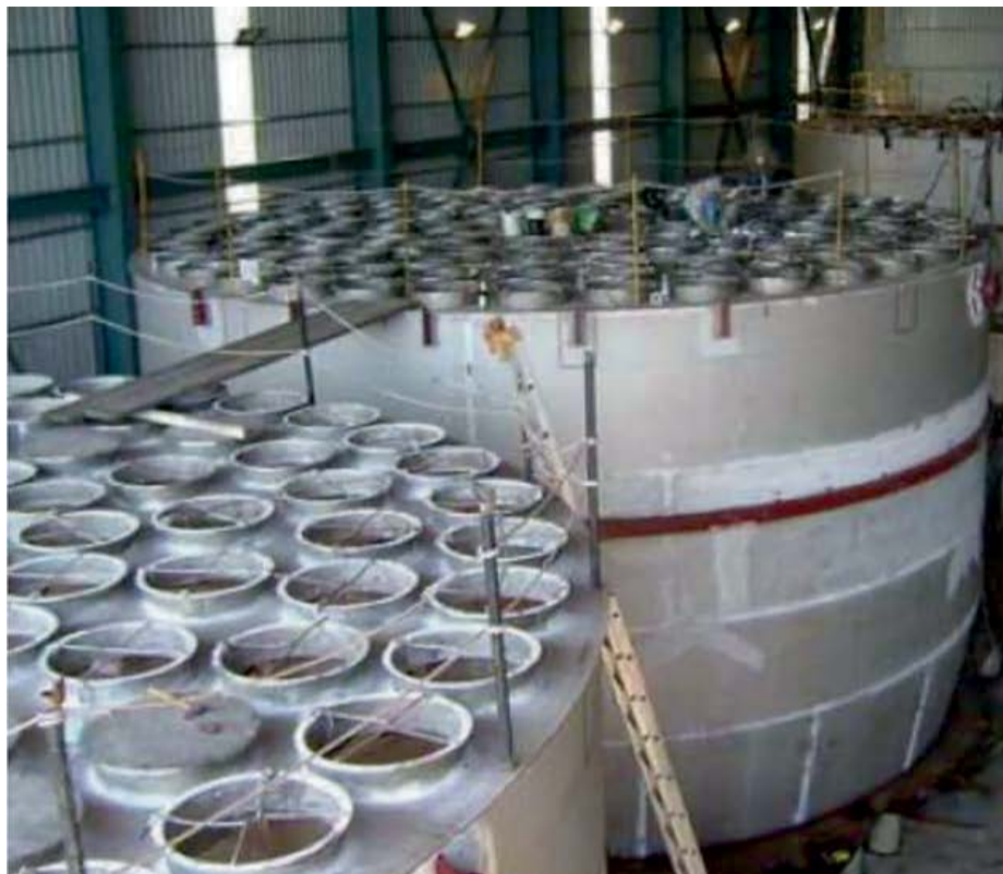
Fig. 7: Shop fabrication of absorption tower parts and transportation of the complete upper portion.
