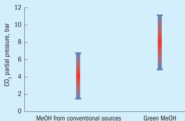
Fig. 15: Typical CO 2 partial pressures in the methanol converter
