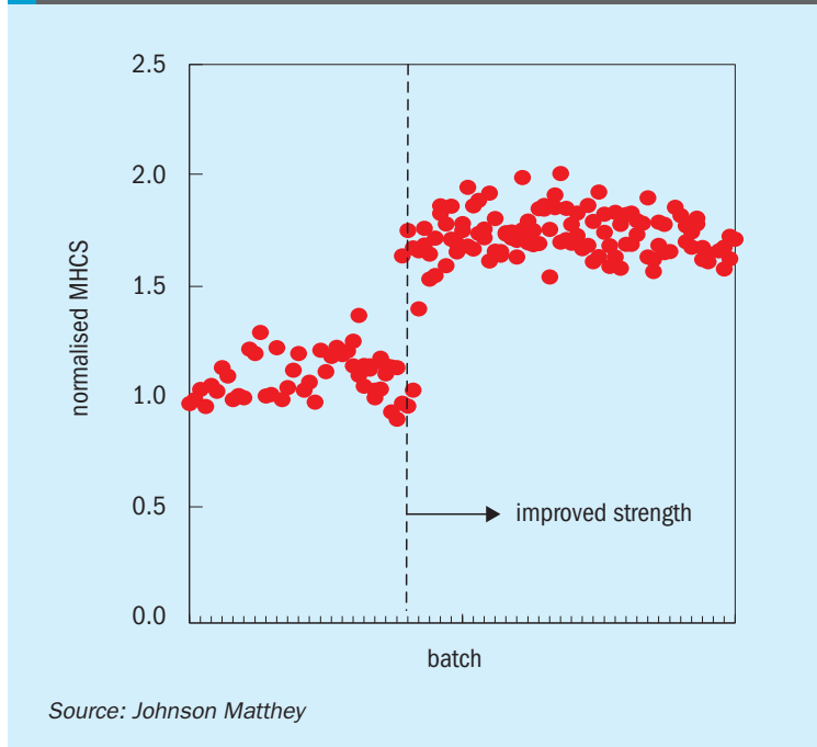
Fig. 7: Normalised mean horizontal crush strength for KATALCO 51-series catalysts
