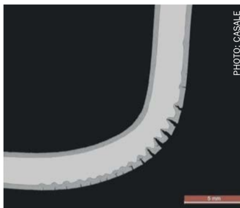
Fig. 1: Effect of increasing penetration of nitriding (darker layer) due to cracks in a thin bended plate.
