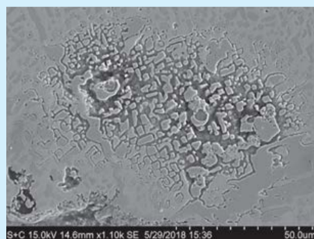
Fig. 1: Metal dusting attack on a 25Cr35NiNbTi (HP-Nb MA) sample – surface “pitting” (left); internal corrosion, SEM image transversal section (right)
