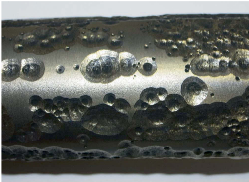
Fig. 1: Alloy 601 showing metal dusting pits.
