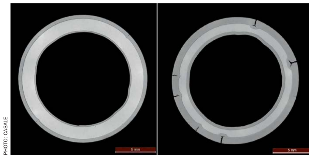
Fig. 5: Nitrided sections of an interchanger tube. Cracks start at high nitride thickness
