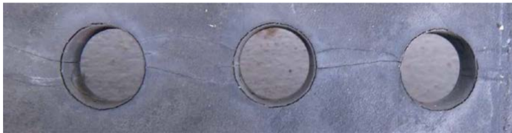
Fig. 3: Effect of nitriding in a 20 year old perforated plate.
