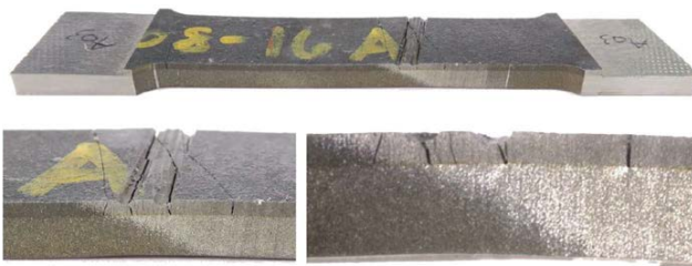
Fig. 2: Nitrided sample after traction test. Cracks occurred in the nitrided layer
