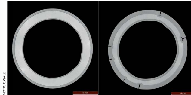
Fig. 5: Nitrided sections of an interchanger tube. Cracks start at high nitride thickness
