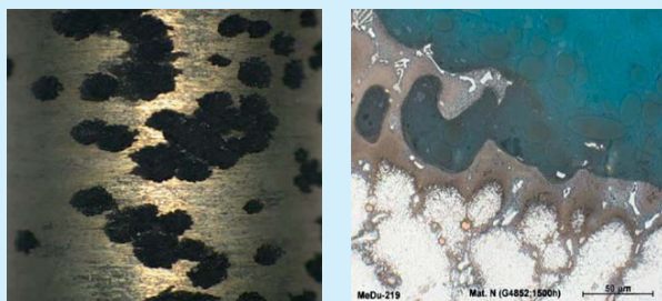
Fig. 7: Metal dusting trials on alloy Centralloy® G 4852 Micro
