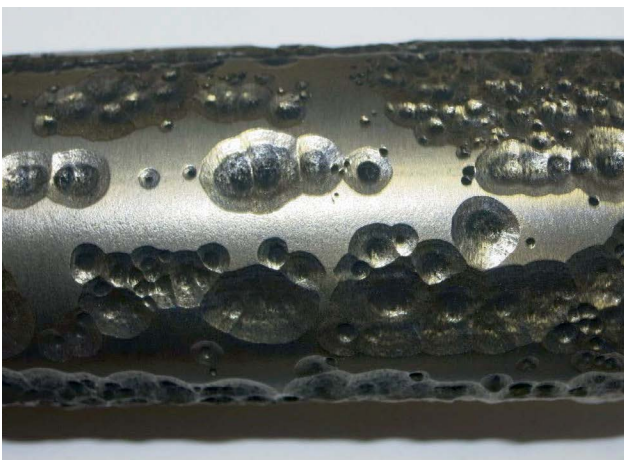
Fig. 1: Alloy 601 showing metal dusting pits.
