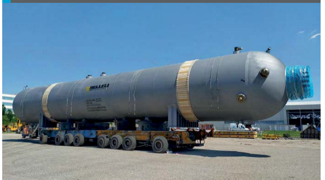
Fig. 4: The Ultra-Low Energy pool reactor for transport to China
