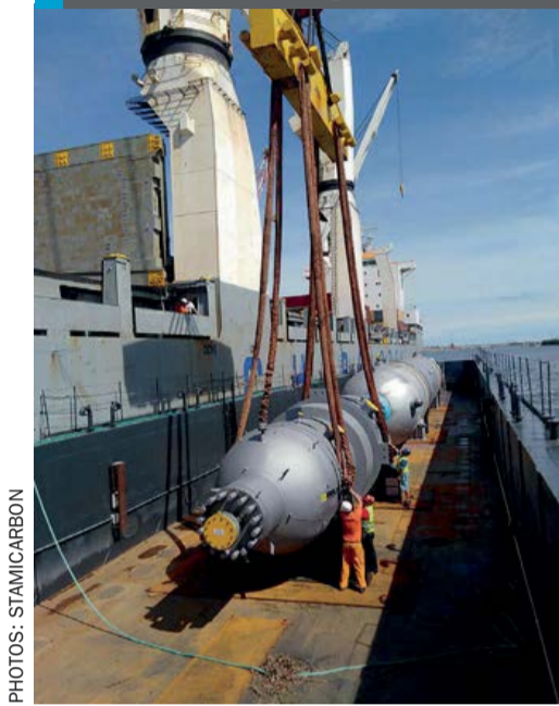
Fig. 3: Stripper and pool reactor for Hubei Sanning, China
