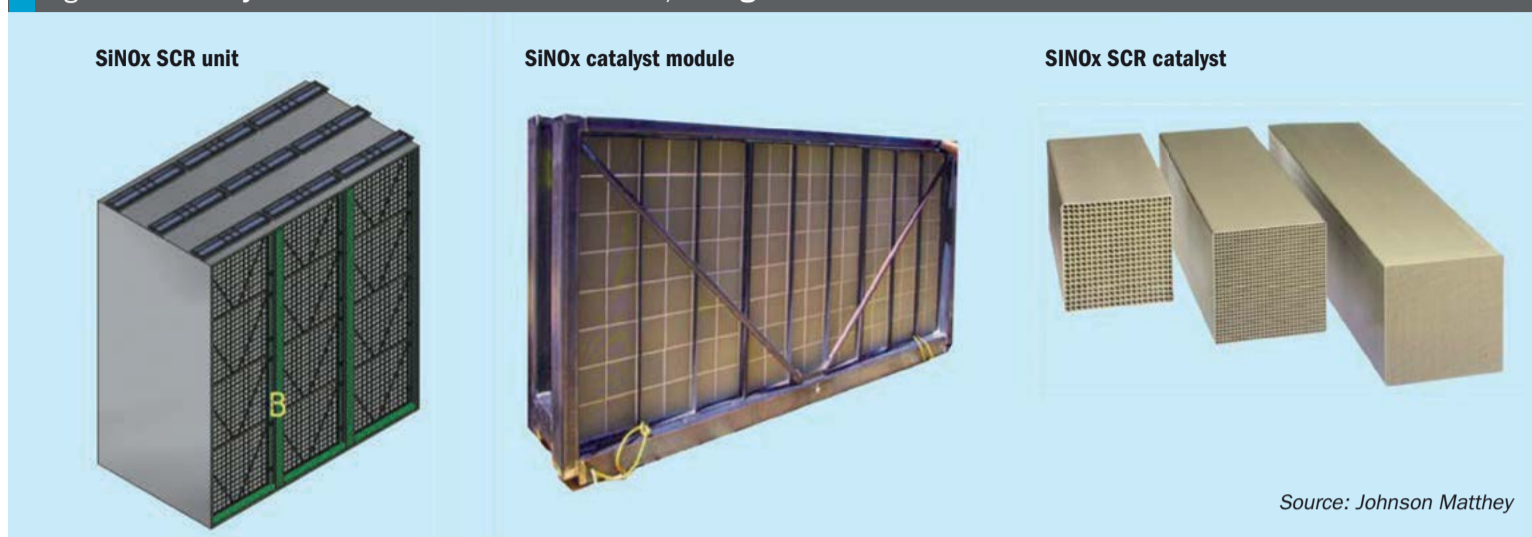
Fig. 6: SCR catalyst is formed as extruded monoliths, arranged in modules to form the SiNOx SCR unit
