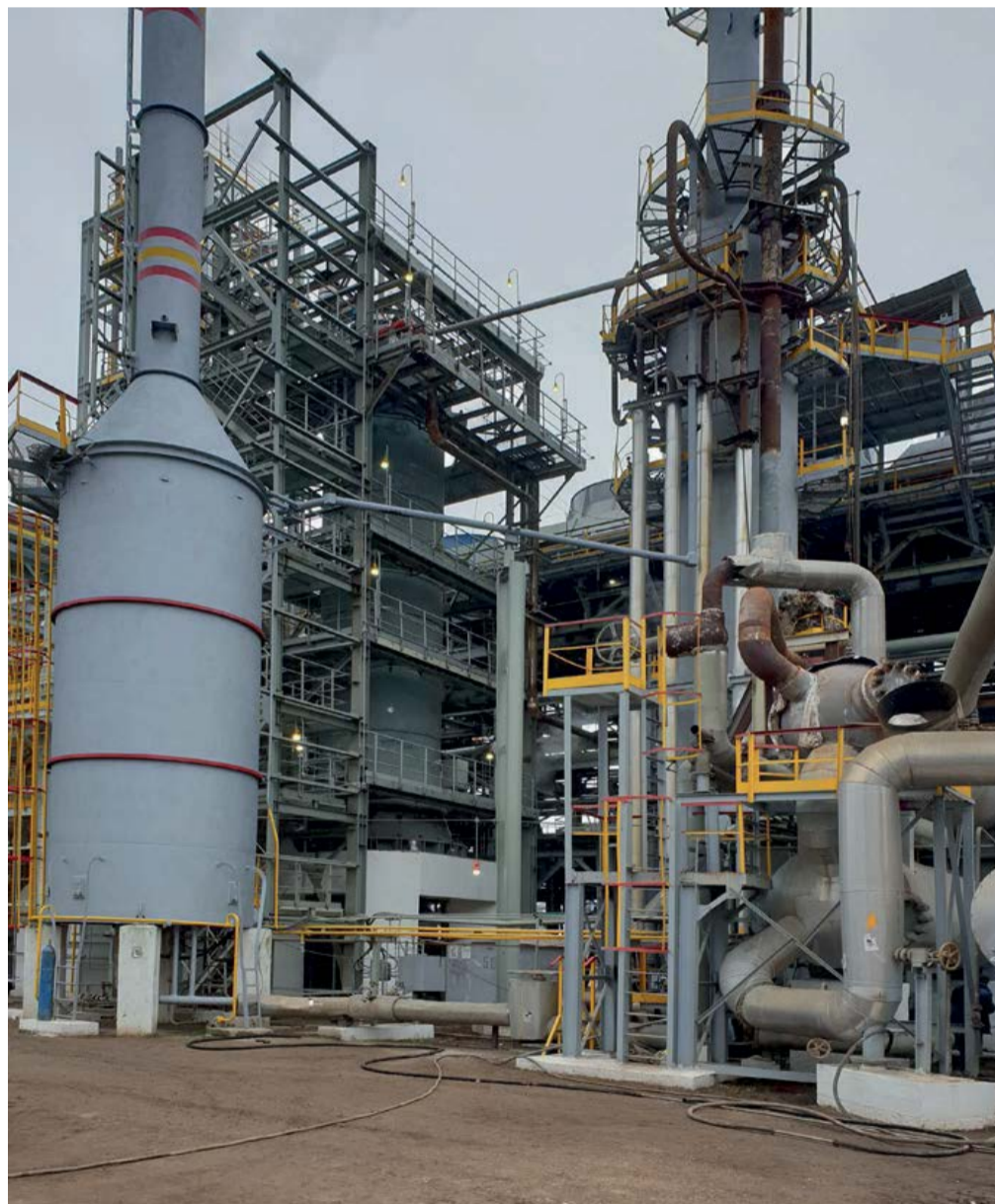
Fig. 4: Add-on ammonia converter.
