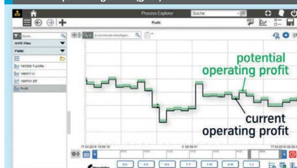
Fig. 18: Screen view of the calculated profitability of the actual plant (black) and the optimised digital twin (green)
