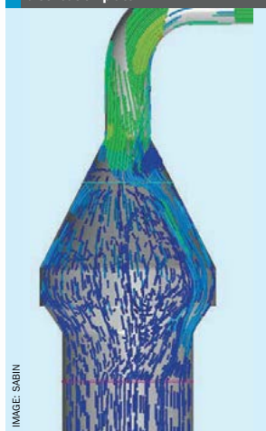
Fig. 13: CFD simulation with additional distribution plate
