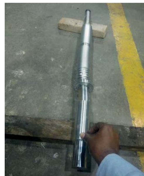
Fig. 2: Bend in valve stem.
