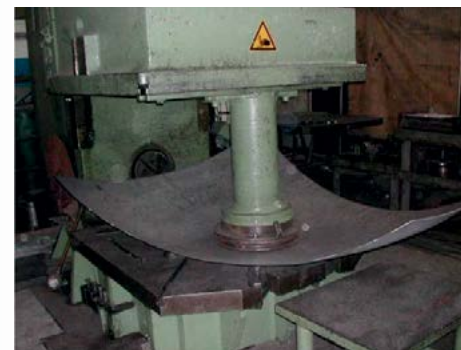
Fig. 8: Forming of a spherical lining segment on a press.
