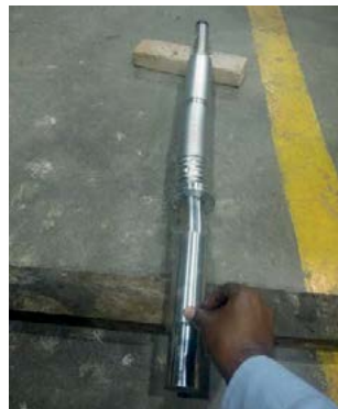
Fig. 2: Bend in valve stem.
