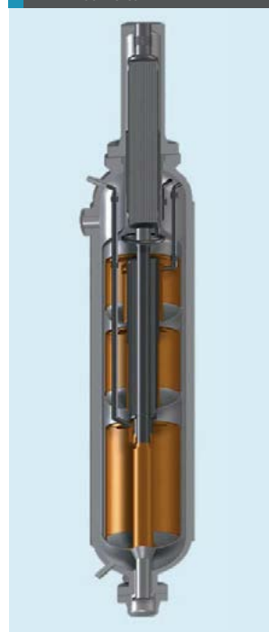
Fig. 10: Revamping of a bottle shape converter
