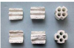
Fig. 5: Q-shape broken showing resultant large pieces having small impact on pressure drop.
