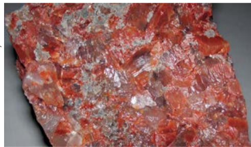
Permian-age potash-bearing rock, Carlsbad potash mining district, Eddy County, New Mexico. Potash ore needs to be crushed and ground to liberate the target mineral sylvite from unwanted halite.
