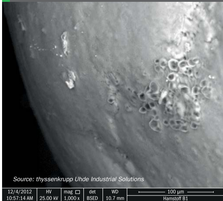
Fig. 1: Electron microscope image of a PLA-coated fertilizer granule
