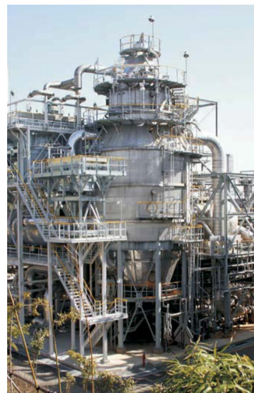
Fig. 4: Ammonium sulphate reactive crystalliser.
