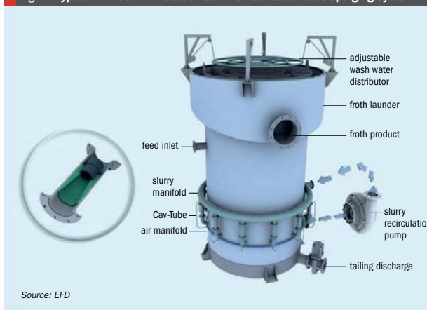
Fig. 1: Typical EFD column flotation cell with cavitation-tube sparging system
