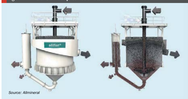
Fig. 1: Allmineral's allflot ® pneumatic flotation machine
