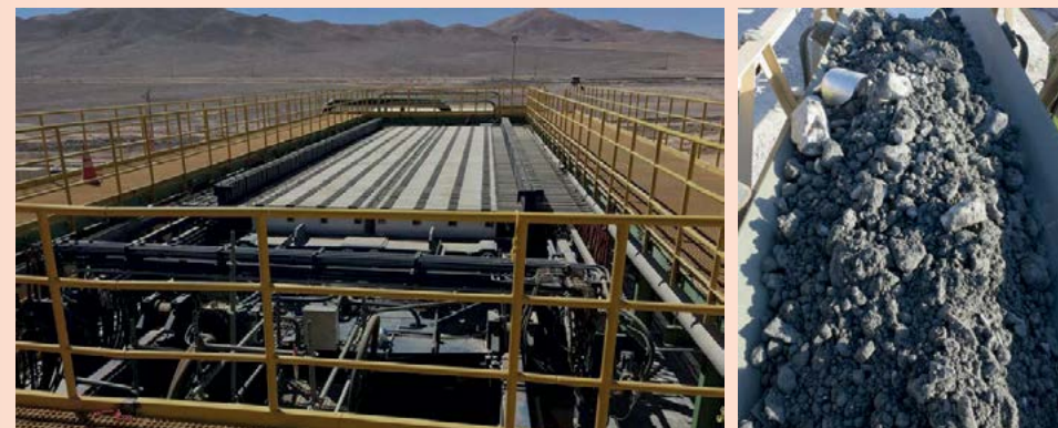
Above left: Colossal filter demo plant. Above right: Stable GeoWaste generated by the EcoTails process.
