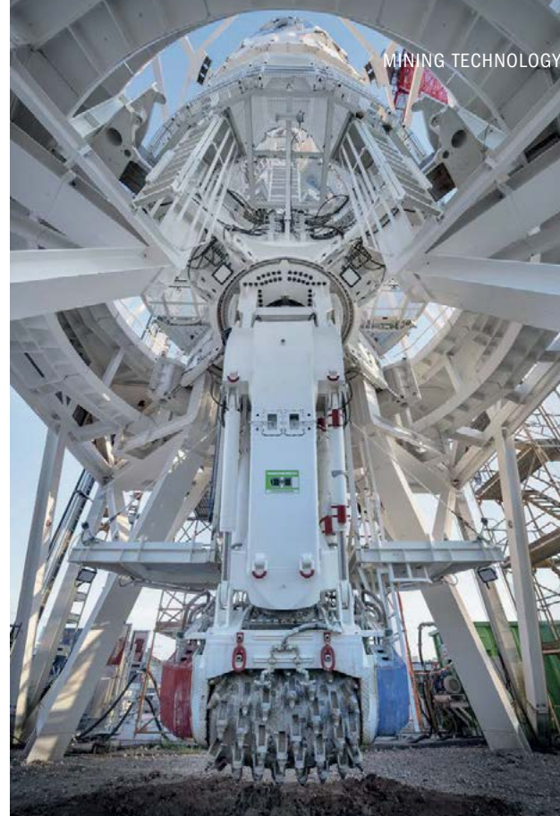
Sirius Minerals Herrenknecht shaft boring roadheader.
