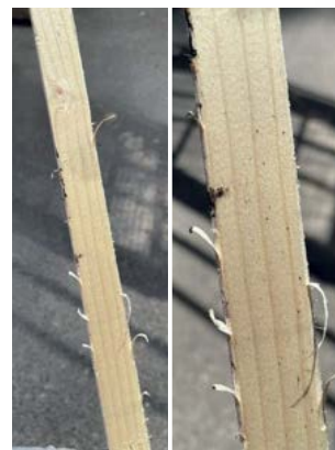
Fig. 5: Clean stick test results from J. R. Simplot's IPAT installation of PI fibre beds at 18 months of service.
