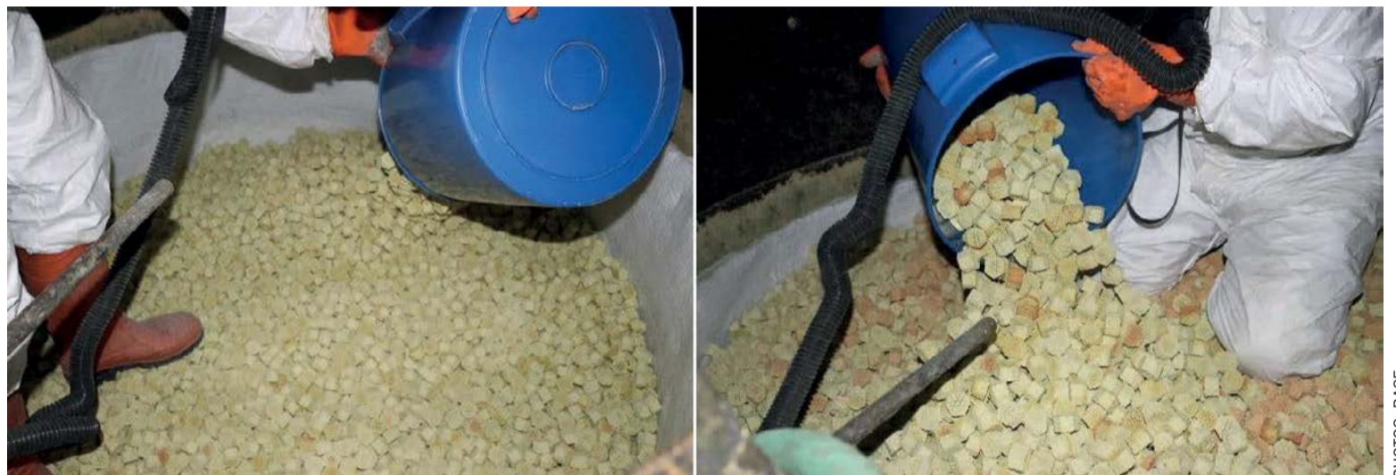
Fig. 3: Filling of the O4-115 X3D™ catalyst into bed 3 of the converter at the BASF reference plant.
