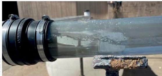
Left: Example of liquid level rise at entrance to horizontal elbow fitting. Right: Example of liquid level viewed through sight glass on elbow.
