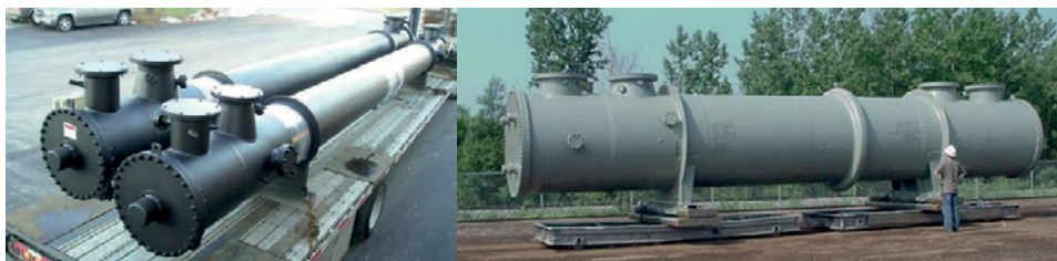
Fig. 3: The increasing size of acid coolers. Left: 800 t/d plant, 0.8 m shell ID, 5.3 m³ acid, 2.4 m³ water. Right: 4,400 t/d plant, 1.8 m shell ID, 18 m³ acid, 7.5 m³ water.
