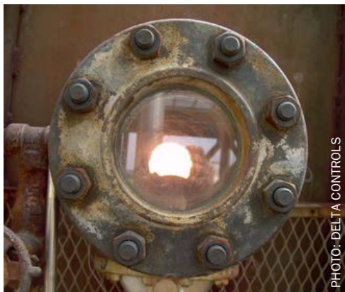
Fig. 1: Traditional sight ports are ubiquitous but suffer from blockage, glass occlusion and a limited view.
