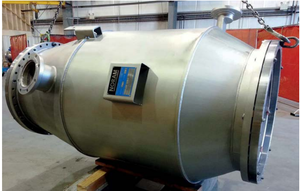
NORAM's patented acid entrainment mitigation device (EMD).
