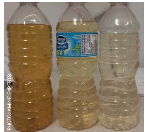
Fig. 8: Increasing clarity of continuously-circulating cold water as wash progressed.
