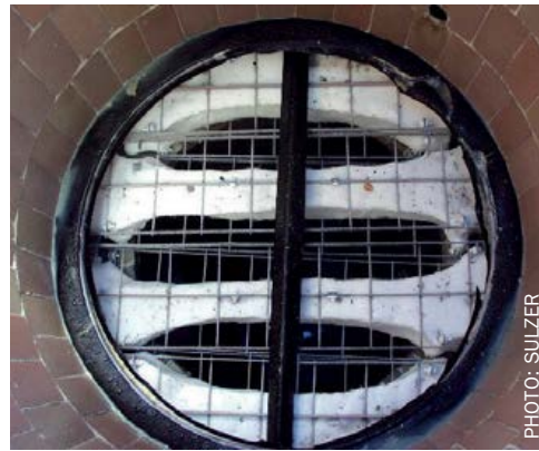
Fig. 5: Shrunken fluoroplastic wire mesh mist eliminator which was exposed to a temperature of ~120°C.
