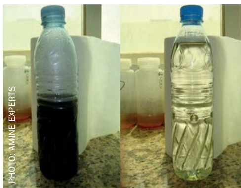
Fig. 5: First (left) and last (right) circulating amine-wash solution samples.
