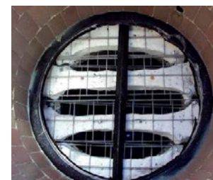
Fig. 5: Shrunken fluoroplastic wire mesh mist eliminator which was exposed to a temperature of ~120°C.
