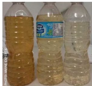
Fig. 8: Increasing clarity of continuously-circulating cold water as wash progressed.
