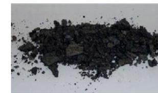
Fig. 4: No. 1 reheater process (shell) side deposits.
