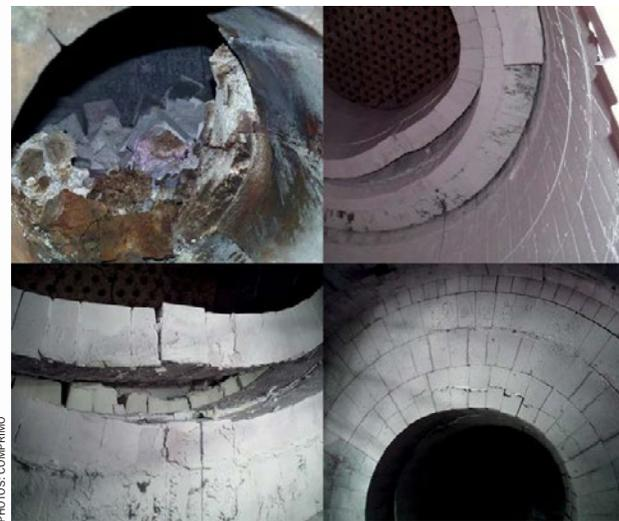
Fig. 7: Thermal reactor damage from liquid hydrocarbon carryover.
