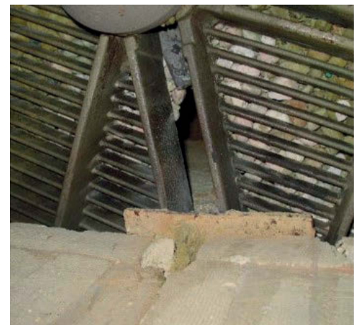
Fig. 4: Shifting grids leading to gas bypass and catalyst drop.
