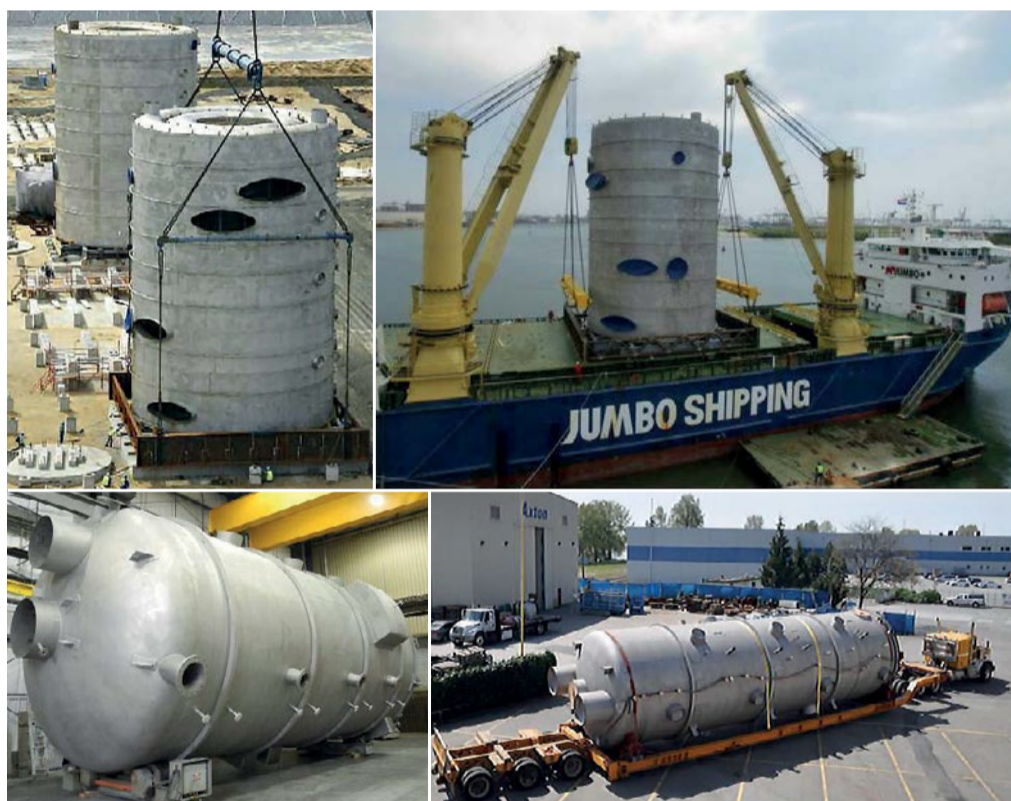
Fig. 1: Examples of converters assembled at fabrication shop, shipped in one piece, and lifted into place.
