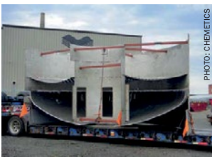
Fig. 11: Chemetics converter module delivery.
