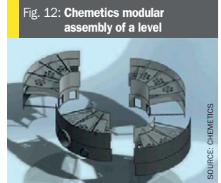
Fig. 13: Two half ring modules per level for smaller converters.
