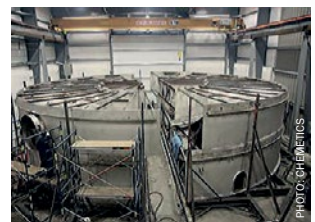
Fig. 13: Two half ring modules per level for smaller converters.
