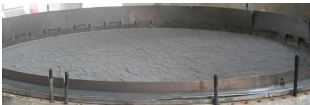
PGM catalyst in a nitric acid plant.
