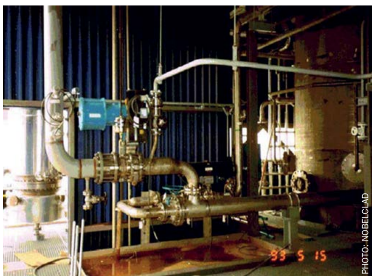
Fig. 2: Grande Paroisse pipe reactor at DSM Geleen (now OCI).
