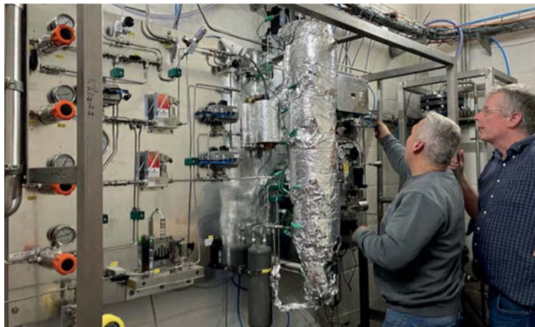
Fig. 1: High-pressure ammonia cracking facilities at the high-pressure laboratory at the University of Twente, the Netherlands.
