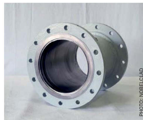
Fig. 6: Tantalum test spool.
