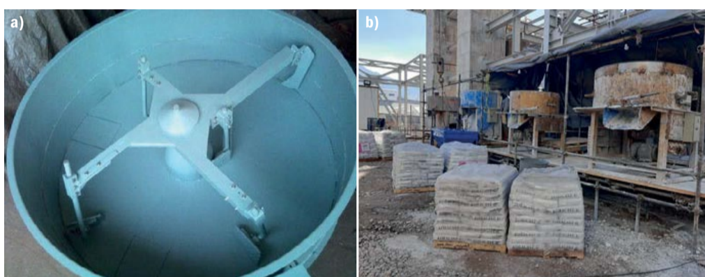
Fig. 5: a) Puddle-type mixer; b) Arrangement of four used puddle mixers.
