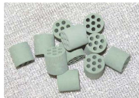
Fig. 2: Leading secondary N 2 O abatement catalyst Yara 58-Y1.
