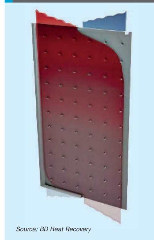
Fig. 3: Counter flow heat exchanger
