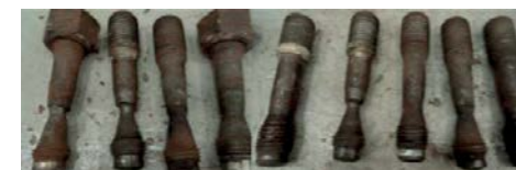
Fig. 6: Corroded carbon steel bolts.
