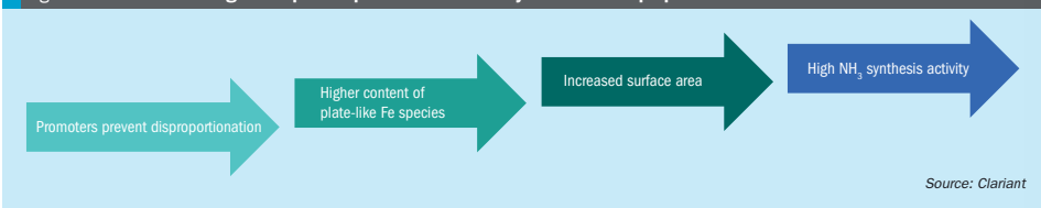
Fig. 5: Scheme illustrating the impact of promoters on activity based on the proposed reduction mechanism
