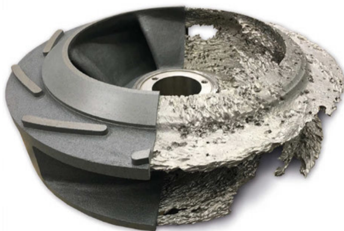
A half repaired pump impeller refurbished (left) using Düchting's unique SIConit refurbishment process.
