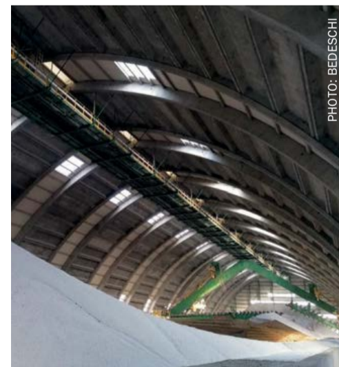
A Bedeschi 2,400 t/h fertilizer reclaimer installed at OCP's Jorf Lasfar complex in Morocco.
