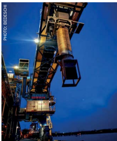
The Bedeschi 1,000 t/h fertilizer shiploader installed at PT Petrokimia Gresik's Demarga jetty in Indonesia.
