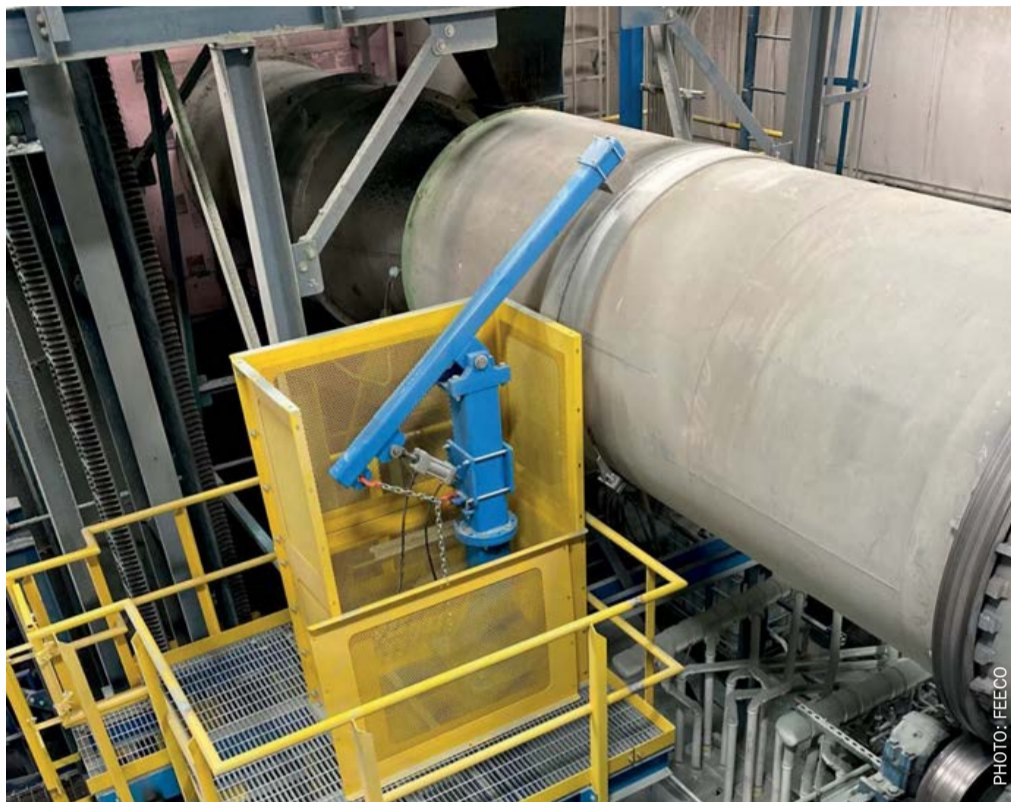
A pneumatic hammer knocker mounted on the side of a rotary dryer.
