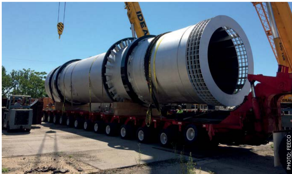
Trommel screen ('grizzly') at the discharge end (right) of rotary dryer.
