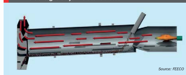
Fig. 1: Co-current dryer illustration: material, hot air, and combustion products all move through the dryer in the same direction
