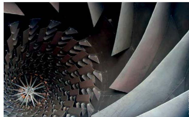
Interior view of a rotary dryer with flights.
