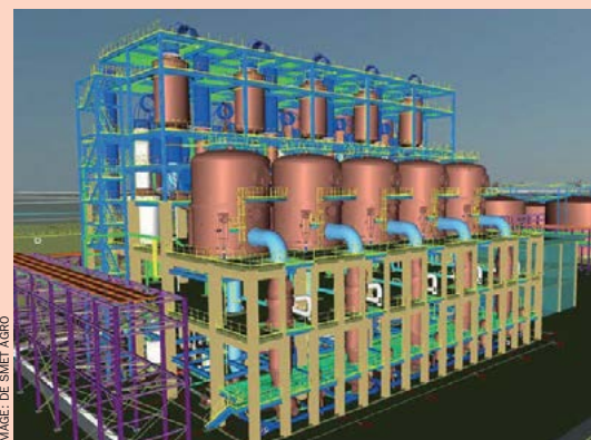
Left: 3D model of the concentration section of the proposed phosphoric acid plant for the Ammaroo phosphate project.
