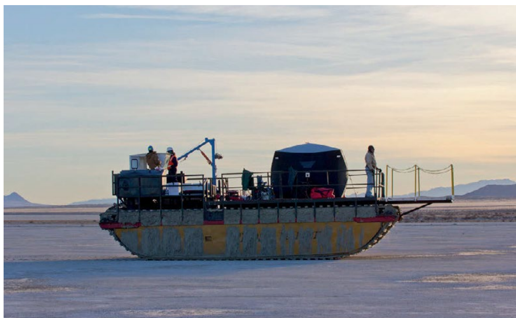
Trenching machine, Sevier Playa, Millard County, Utah.
