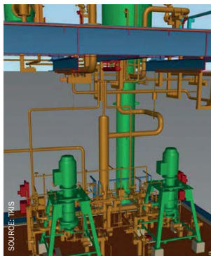
Fig. 1: Self-regulating transfer pump for urea melt: typical setup.
