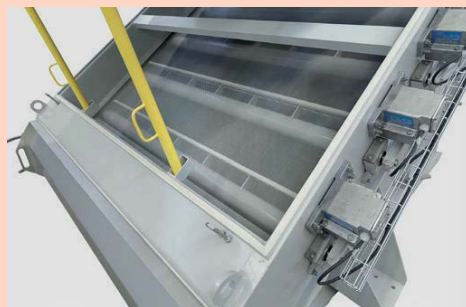
Vibrating screen on RHEWUM's RHEsono screening machine.
